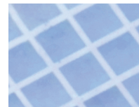
Close-up of CdWO 4 2D array with diffuse reflector technology.
