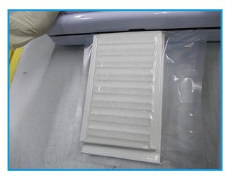
The vacuum sealed package is placed in a plastic box with top & bottom support as shown.
