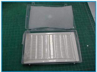
The plastic box is vacuum sealed & marked with tape bearing CsI(TI).
