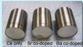
Fig. 1 Photo of \phi 60 mm x 80 mm LaBr 3 :Ce scintillation detectors
