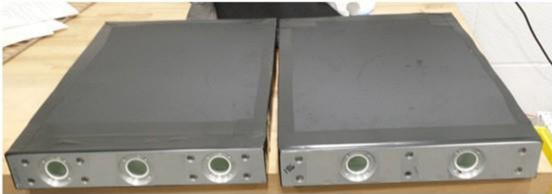
New prototypes with hermetically sealed with optical windows
